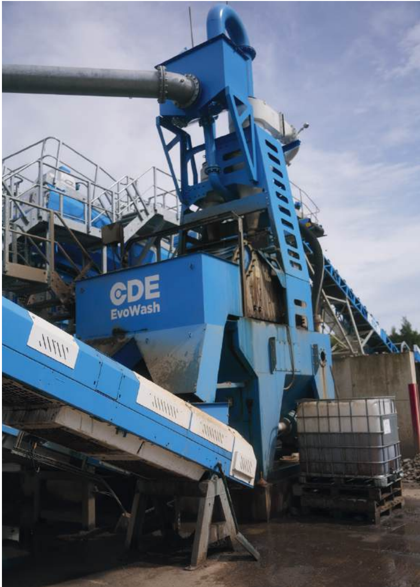
CDE's compact EvoWash sand washing system integrates a dewatering screen, sump and hydrocyclone configuration
